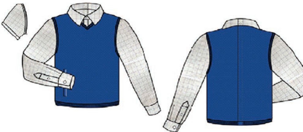
This design is a dress shirt with a built-in sweater vest, center-back opening, a right side slit to provide access to a gastrostomy tube and a sewn-in cotton undershirt. It also features interchangeable short and long sleeves. The idea of consolidating several features into one was to facilitate caregiver dressing.
